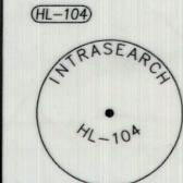
FOUND: 1/2" REBAR WITH A 1" DIA. AL. CAP MARKED AS SHOWN. PROJECTING ±0.5' ABOVE THE GROUND. POINT IS ±6' NORTH OF RIM OF CLIFF WITH REMNANTS OF AERIAL TARGET MATERIAL.
