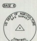
SET: USFS STANDARD ROD MONUMENT, A 2-1/2" DIA. AL. CAP MARKED AS SHOWN, FLUSH WITH THE GROUND, RAISED A ROCK COLLAR. CONTROL POINT IS NEAR RIM OF CLIFF.
