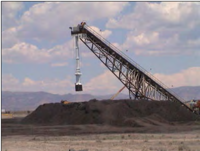
Photo 3: Raw material conveyor and radial stacker with telescoping chute to reduce emissions.
