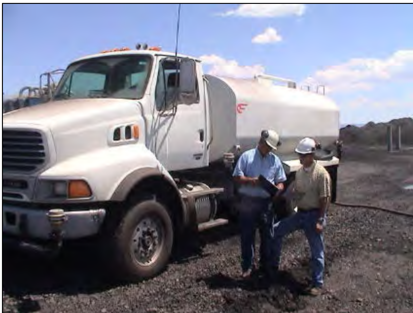
Photo 9: Water truck used daily for dust suppression on roads.
