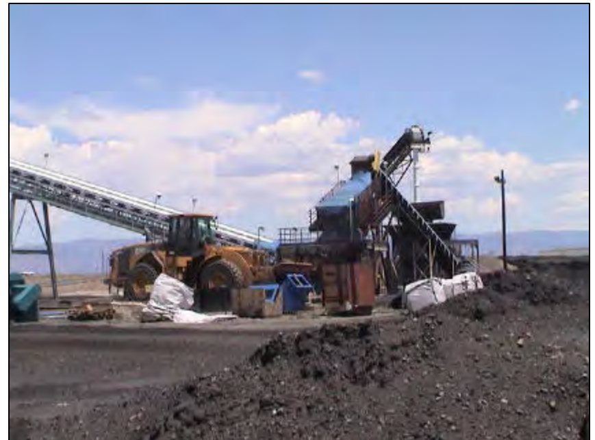
Photo 4: Feed hopper, conveyor, screen and hammermill – covered to reduce emissions.
