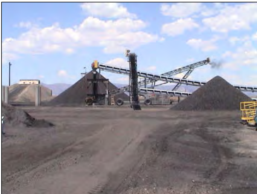
Photo 7: Conveyors and stackers for final coal piles.
