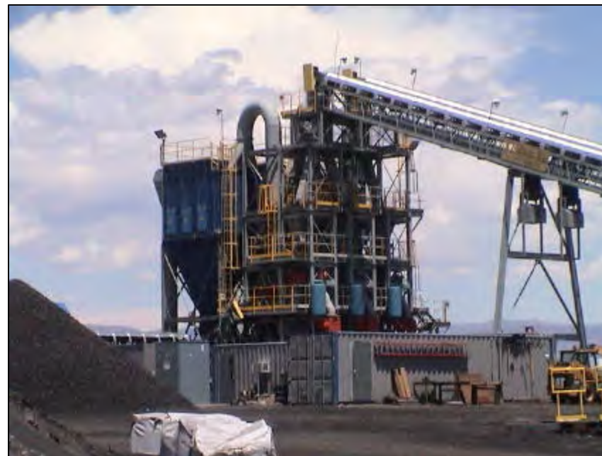
Photo 6: Coal separation and bag house dust control equipment.
