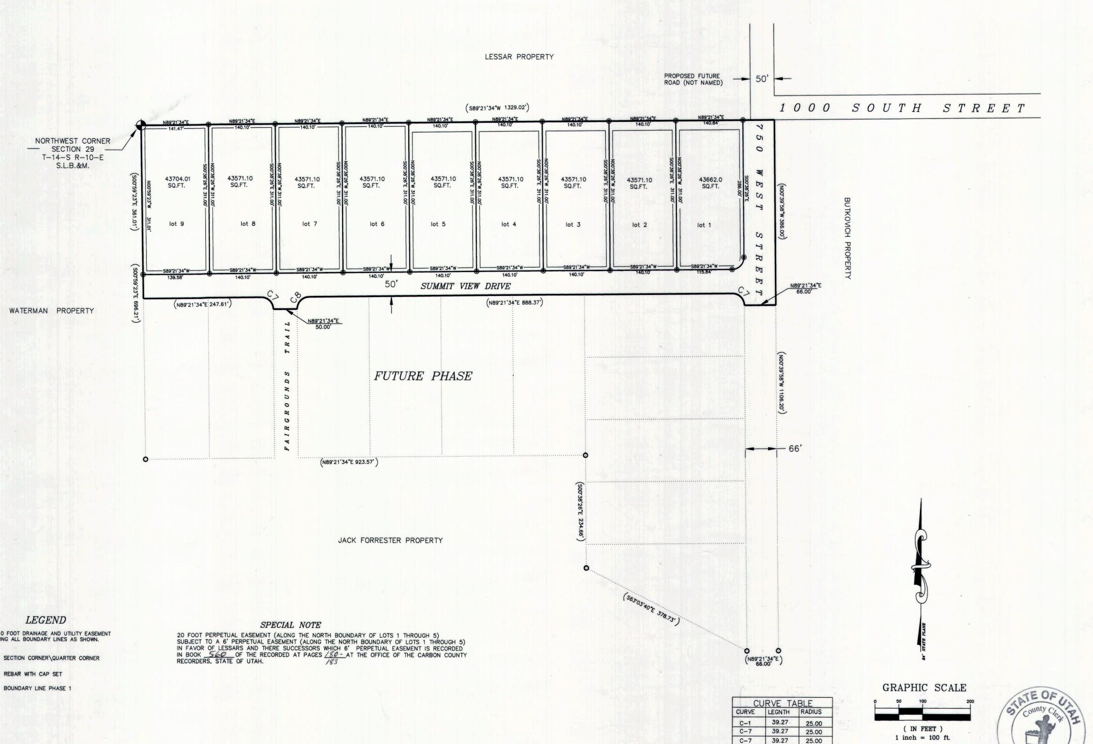
A 10 FOOT DRAINAGE AND UTILITY EASEMENT ALONG ALL BOUNDARY LINES AS SHOWN.
