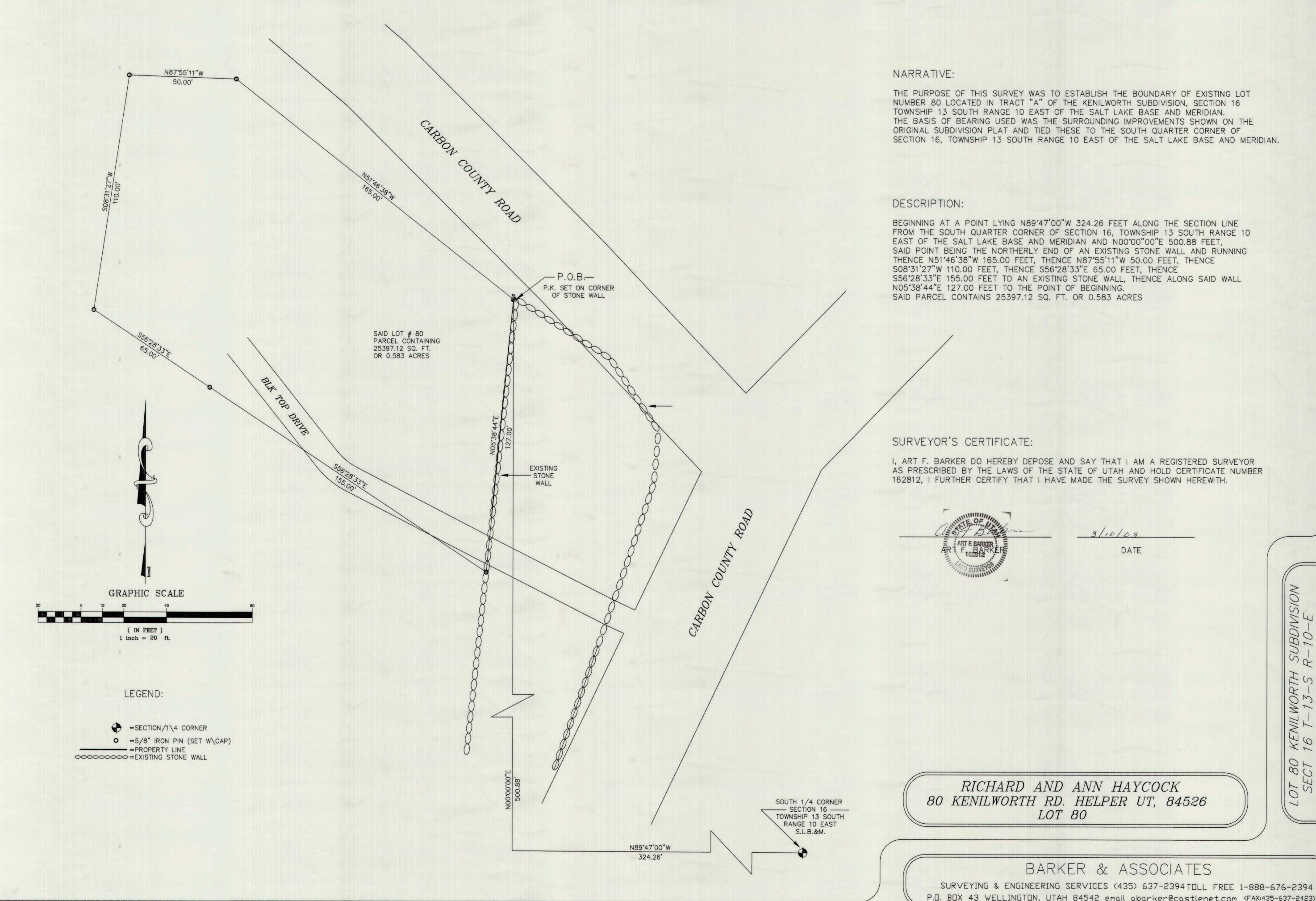
THE PURPOSE OF THIS SURVEY WAS TO ESTABLISH THE BOUNDARY OF EXISTING LOT NUMBER 80 LOCATED IN TRACT "A" OF THE KENILWORTH SUBDIVISION, SECTION 16 TOWNSHIP 13 SOUTH RANGE 10 EAST OF THE SALT LAKE BASE AND MERIDIAN. THE BASIS OF BEARING USED WAS THE SURROUNDING IMPROVEMENTS SHOWN ON THE ORIGINAL SUBDIVISION PLAT AND TIED THESE TO THE SOUTH QUARTER CORNER OF SECTION 16, TOWNSHIP 13 SOUTH RANGE 10 EAST OF THE SALT LAKE BASE AND MERIDIAN.
